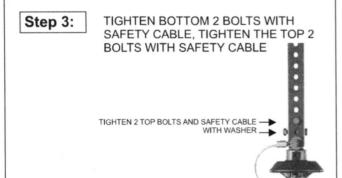
TIGHTEN 2 BOTTOM BOLTS & -SAFETY CABLE WITH WASHER \_ TIGHTEN 2 TOP SET SCREWS WITH
